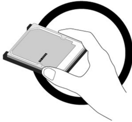
Figure 11. HDD handling guide - Do not Touch Cover and PCB!
