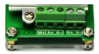
The tester has four jacks which connect with M+/A+/A-/V+/V-. A+ and A- ports are connected with the positive and negative poles of the test objects, working as the current channel in discharging. V+ and V- ports are connected with the positive and negative poles of the test objects, working as the voltage channel in voltage tests. This way of using four individual cables will help eliminate the effect of wires on the test result and improve the test precision.
